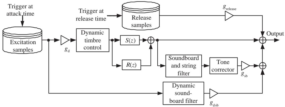
Figure 7: Block diagram of the waveguide synthesis algorithm for the harpsichord with dynamics modeling.
