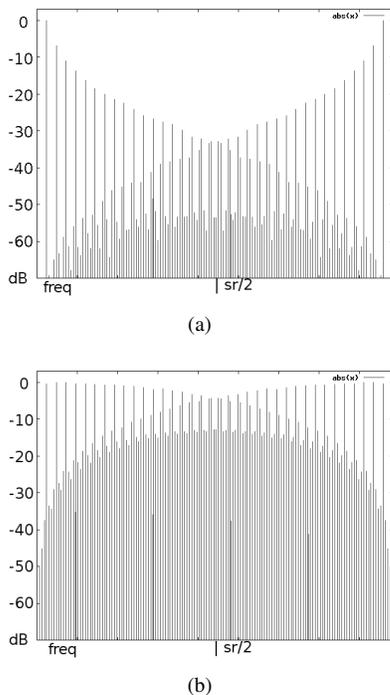
Figure 4: (a) The spectrum of the resynthesized sawtooth, based on the integrated wave-table method. (b) The hardest case: a resynthesized noise wave-table.
