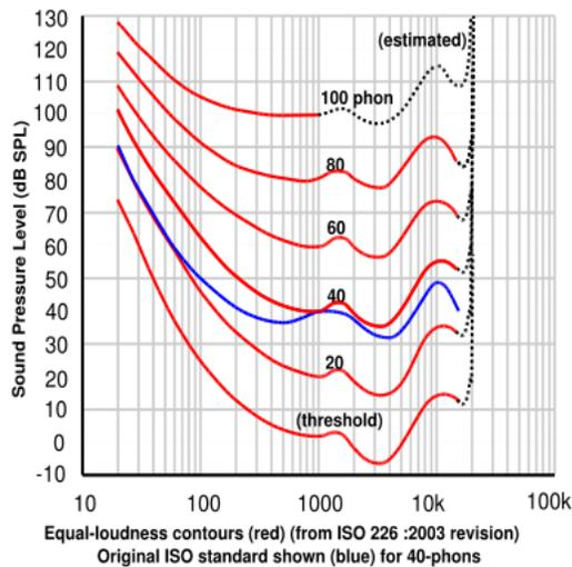
Figure 5: Curves of equal loudness (diagram from wikipedia) suggest that aliasing that occurs above 15 kHz only has a limited influence upon the signal frequencies between 200 Hz and 8 kHz are critical.
