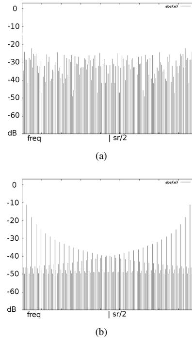
Figure 3: (a) Generating a random periodic waveform from a lookup table of size  $N = 1024$ , frequency  $f_0$  is 1200 Hz. (b) Spectral content of an integrated random lookup table of the same function, the fundamental frequency of 1200 Hz can be recognized.
