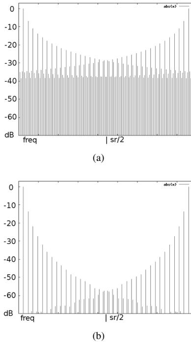
Figure 2: (a) Generating a sawtooth waveform from a lookup table of size  $N = 1024$ , frequency  $f_0$  is 1200 Hz. (b) Spectral content of an integrated lookup table of the same sawtooth.
