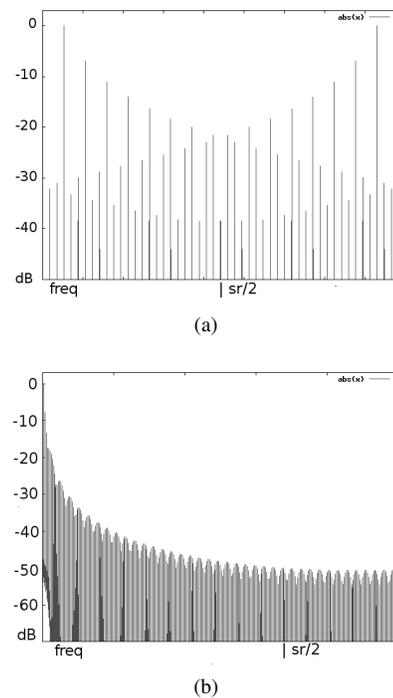
Figure 1: (a) Aliasing through resampling of a wave-table. Partials are mirrored at half the sampling frequency and disturb the original signal. (b) Spectral content of a sawtooth at frequency 44100/1024, the amplitude at half sampler-rate is about 54 dB lower.
